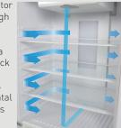
shelves at each shelf level. A uniform freezer temperature is maintained through a cold wall refrigeration system with natural circulation.
